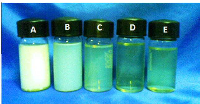
Fig. 7. Visual appearance of emulsion. A - Coarse emulsion before sonication, B - 1:1 (v/v) ratio of basil oil nanoemulsion, C - 1:2 (v/v) ratio of basil oil nanoemulsion, D - 1:3 (v/v) ratio of basil oil nanoemulsion, E - 1:4 (v/v) ratio of basil oil nanoemulsion.
