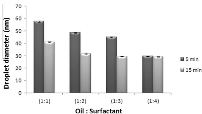
Fig. 8. Effect of sonication time on droplet diameter of emulsion.
