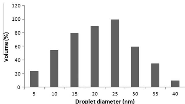
**Fig. 2.** Droplet size distribution of basil oil nanoemulsion with 1:3 (v/v) ratio of oil and surfactant.
