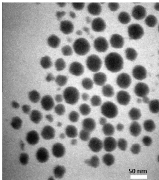
**Fig. 3.** Transmission electron micrograph of basil oil nanoemulsion with 1:3 (v/v) ratio of oil and surfactant.
