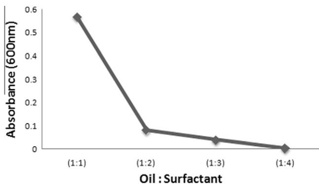
Fig. 6. Effect of surfactant concentration on turbidity of nanoemulsion.
