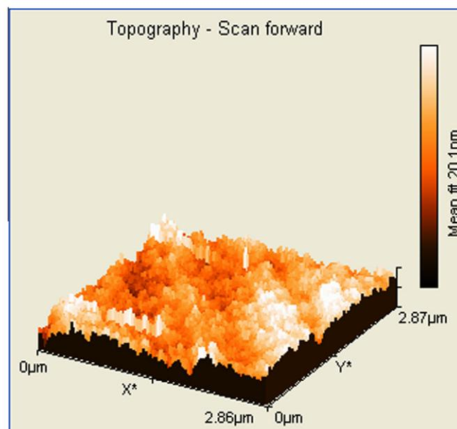
**Fig. 4.** Atomic force micrograph of basil oil nanoemulsion with 1:3 (v/v) ratio of oil and surfactant.
