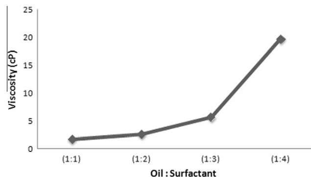
**Fig. 5.** Effect of surfactant concentration on viscosity of nanoemulsion.
