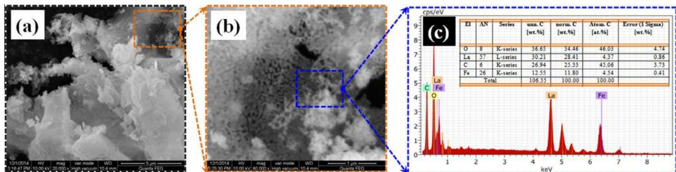
Fig. 2. (a and b) SEM images and (c) the corresponding EDS spectrum of LaFeO<sub>3</sub> catalyst [inset: wt% table].
