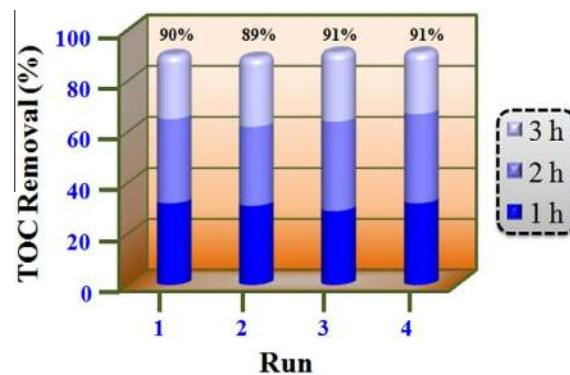
**Fig. 10.** Recyclability test [Experimental conditions:  $\text{LaFeO}_3$  ( $0.5 \text{ g L}^{-1}$ ), 4-chlorophenol ( $1.25 \times 10^{-4} \text{ M}$ ) and KPS (0.5 mmol) were ultrasonicated (40 kHz) for 3 h].
