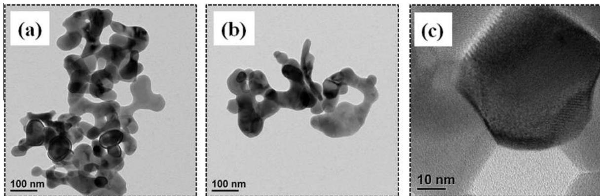
**Fig. 3.** TEM images of  $\text{LaFeO}_3$  catalyst with different magnification (a and b) 100 nm and (c) 10 nm bar scales.
