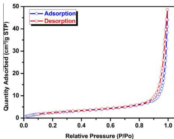
**Fig. 4.**  $\text{N}_2$ -adsorption/desorption isotherm of  $\text{LaFeO}_3$  catalyst.
