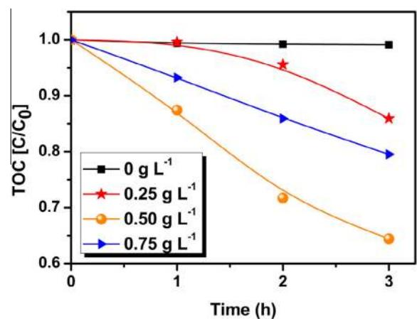
**Fig. 5.** Effect of catalyst dosage [Experimental conditions:  $\text{LaFeO}_3$  and 4-chlorophenol ( $1.25 \times 10^{-4} \text{ M}$ ) were ultrasonicated (40 kHz) for 3 h].
