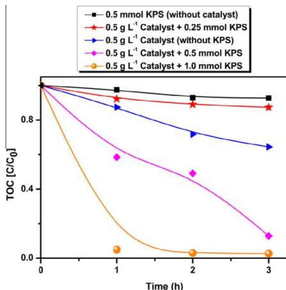
**Fig. 9.** Effect of potassium persulfate (KPS) [Experimental conditions:  $\text{LaFeO}_3$  ( $0.5 \text{ g L}^{-1}$ ), 4-chlorophenol ( $1.25 \times 10^{-4} \text{ M}$ ) and KPS were ultrasonicated (40 kHz) for 3 h].
