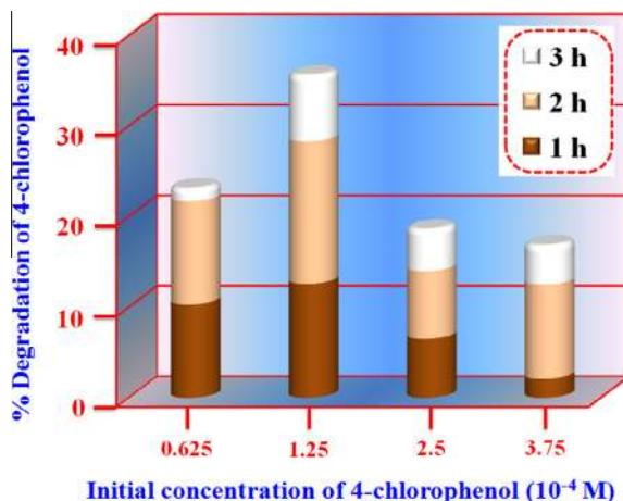
**Fig. 6.** Effect of initial concentration of 4-chlorophenol [Experimental conditions: LaFeO<sub>3</sub> (0.5 g L<sup>-1</sup>) and 4-chlorophenol were ultrasonicated (40 kHz) for 3 h].
