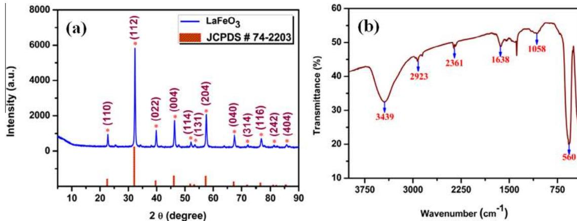
Fig. 1. (a) Powder XRD pattern and (b) FT-IR spectrum of LaFeO<sub>3</sub> catalyst.
