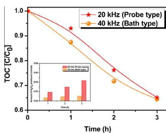
**Fig. 8.** Effect of ultrasound frequency [Experimental conditions: LaFeO<sub>3</sub> (0.5 g L<sup>-1</sup>) and 4-chlorophenol ( $1.25 \times 10^{-4}$  M) were ultrasonicated (20 kHz or 40 kHz) for 3 h] [inset: amount of H<sub>2</sub>O<sub>2</sub> (mmol) produced from each sonicator].
