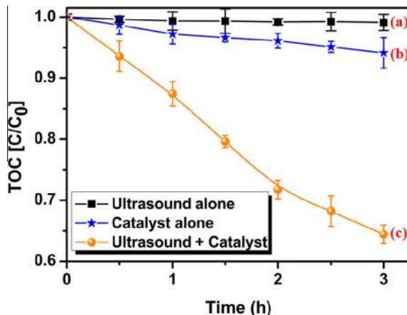
**Fig. 7.** TOC as a function of time [Experimental conditions: (a) 4-chlorophenol ( $1.25 \times 10^{-4}$  M) were ultrasonicated (40 kHz) for 3 h, (b) LaFeO<sub>3</sub> (0.5 g L<sup>-1</sup>) stirred with 4-chlorophenol ( $1.25 \times 10^{-4}$  M) for 3 h and (c) LaFeO<sub>3</sub> (0.5 g L<sup>-1</sup>) and 4-chlorophenol ( $1.25 \times 10^{-4}$  M) were ultrasonicated (40 kHz) for 3 h].
