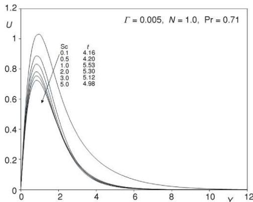
**Figure 5(a). Steady-state velocity profiles at  $X = 1.0$  for different  $Sc$**
