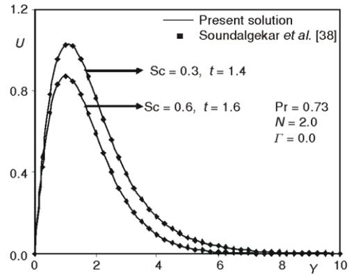
Figure 1(b). Comparison of velocity profiles at  $X = 1.0$
