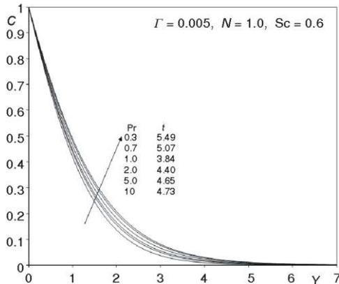
**Figure 4(c) Steady-state concentration profiles at  $X = 1.0$  for different  $Pr$**
