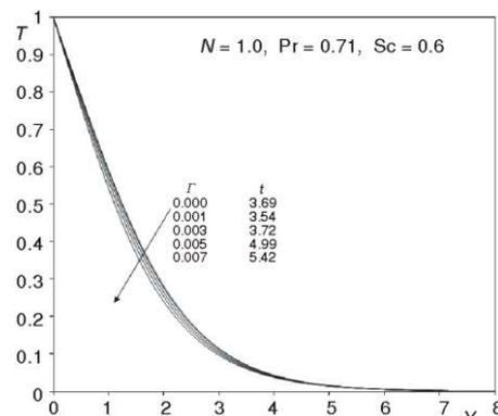
Figure 2(b). Steady-state temperature profiles at  $X = 1.0$  for different  $\Gamma$
