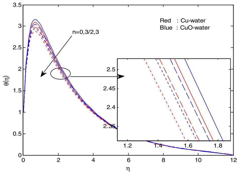
Fig. 18. Variation in temperature profiles for different values of  $n$ .
