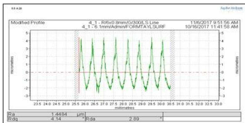
**Figure 4.** A Representative Surface roughness profile.
