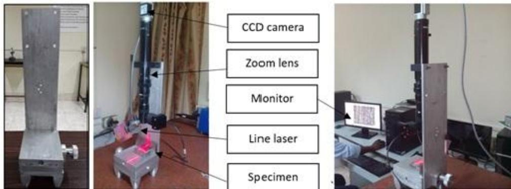
**Figure 5.** The Camera table and the experimental setup.
