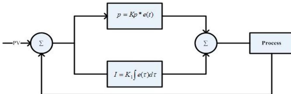
Fig. 4. Block diagram of PI controller.
