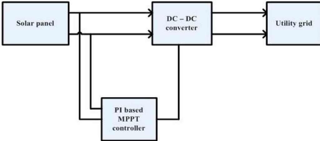
Fig. 2. Overall solar PV panel configuration.
