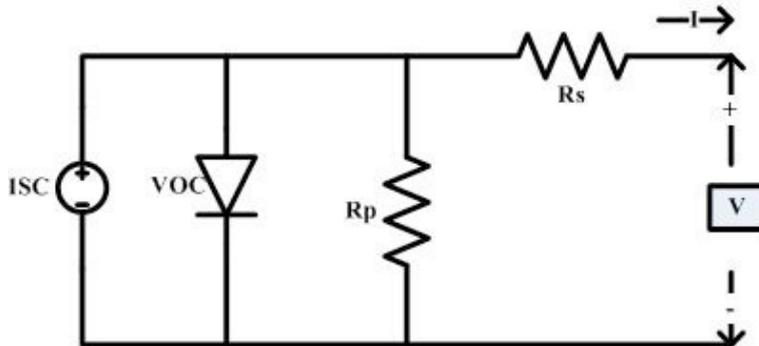
Fig. 3. Equivalent circuit of solar PV panel.
