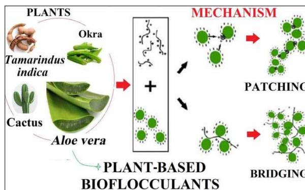
Figure 2 | Mechanism of flocculation using plant-based bioflocculants.
