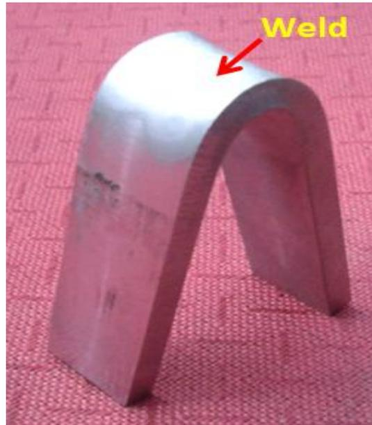
Fig 10. Formability of DSS weld 180° bend
