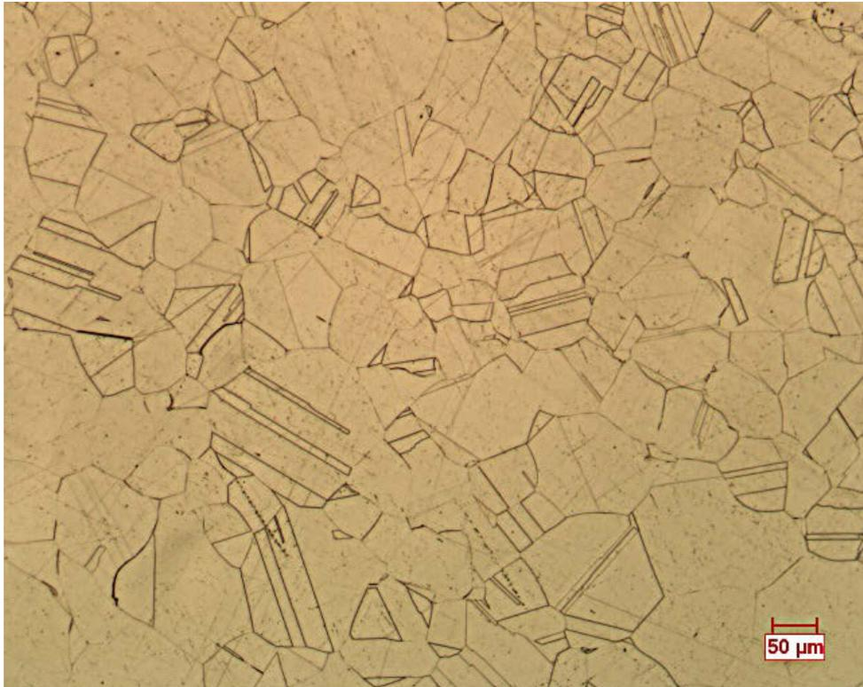
**Figure 1.** Microstructure of Hastelloy C-276 in as-received condition.
