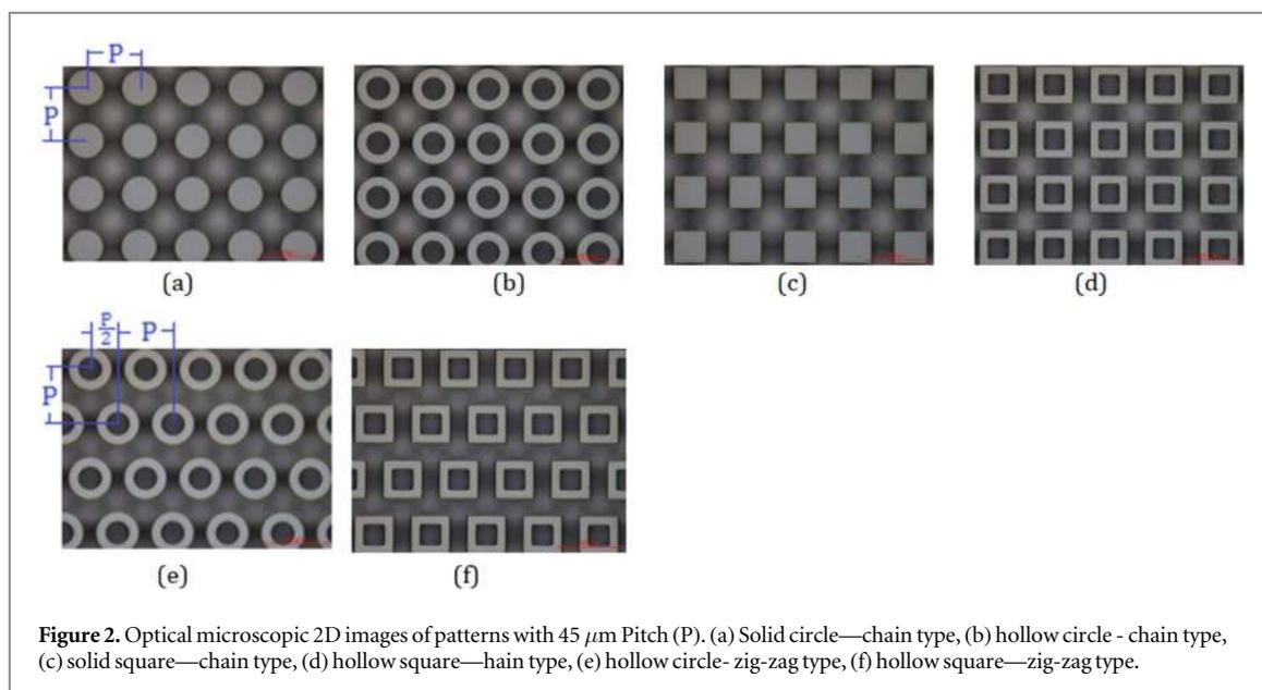
**Figure 2.** Optical microscopic 2D images of patterns with  $45\ \mu\text{m}$  Pitch (P). (a) Solid circle—chain type, (b) hollow circle - chain type, (c) solid square—chain type, (d) hollow square—hain type, (e) hollow circle- zig-zag type, (f) hollow square—zig-zag type.
