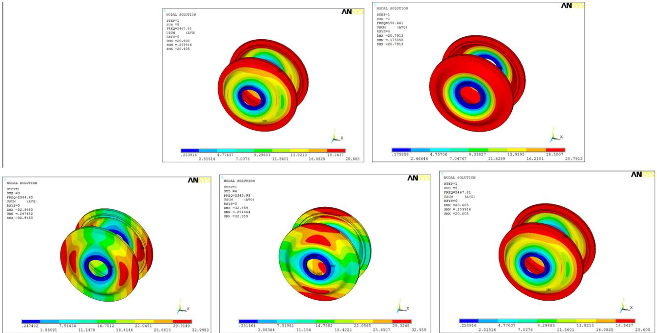
Fig. 24. Rotor casing mode shapes and modal frequencies.
