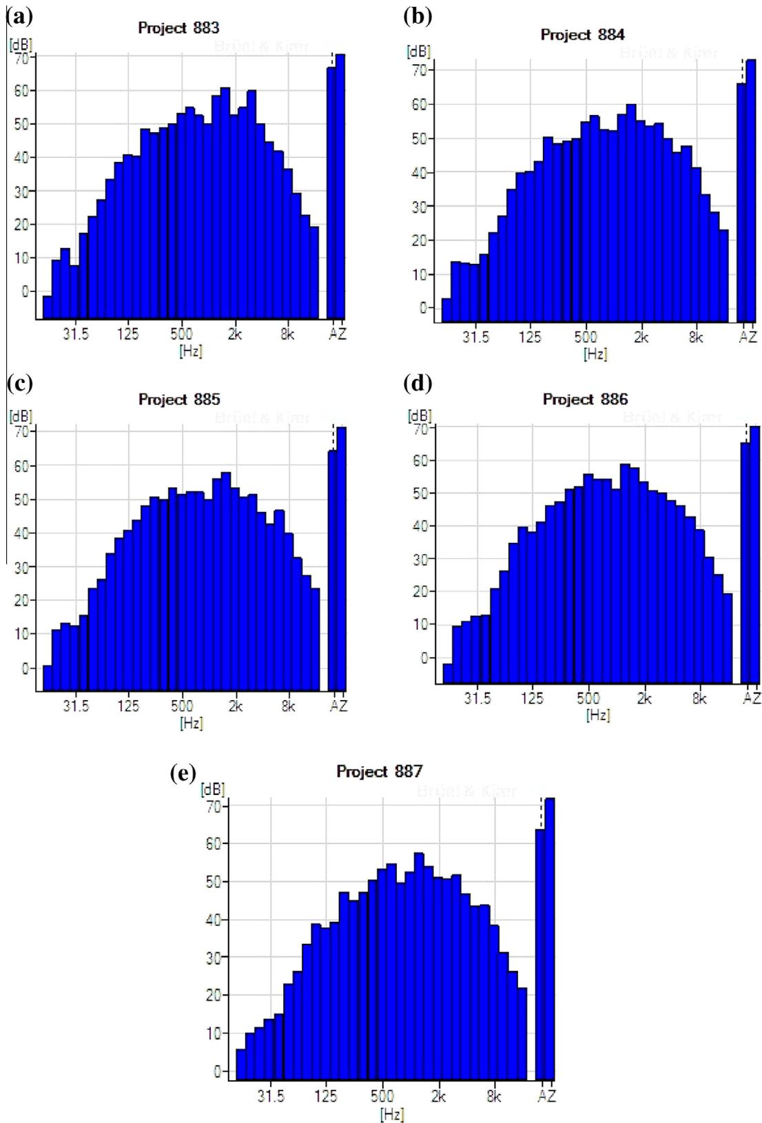
Fig. 31. Noise spectrum for the speed of 1000 RPM at (a) shaft position (b) right side (c) left side (d) opposite to shaft position (e) top position.
