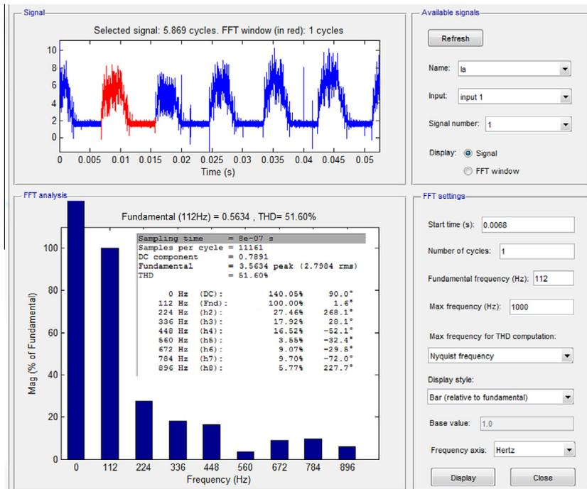
Fig. 25. Measured current waveform and harmonic component of waveform.
