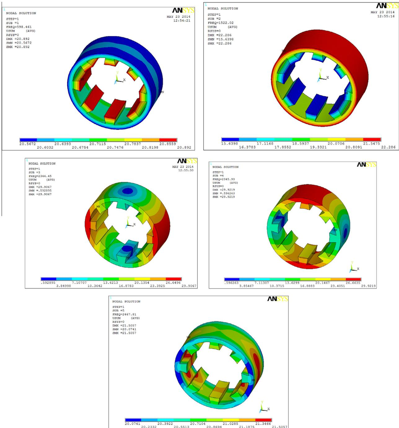
Fig. 23. Rotor lamination mode shapes and modal frequencies.
