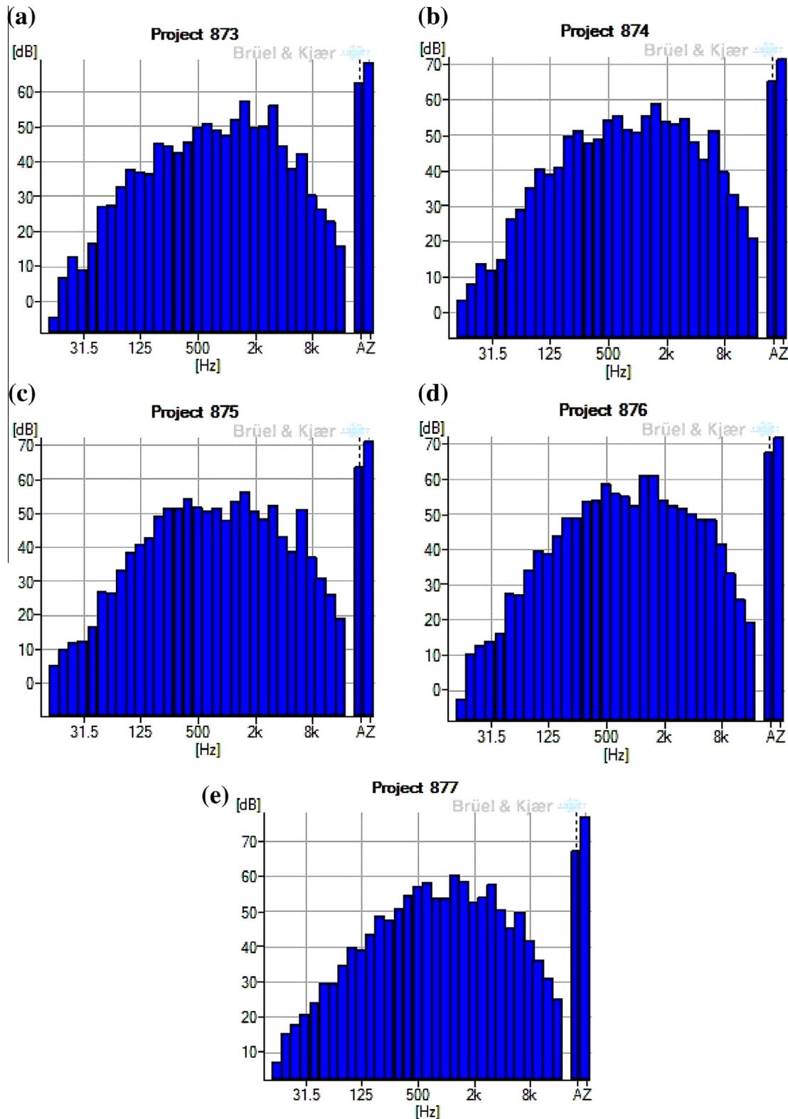
Fig. 29. Noise spectrum for the speed of 250 RPM at (a) shaft position (b) right side (c) left side (d) opposite to shaft position (e) top position.
