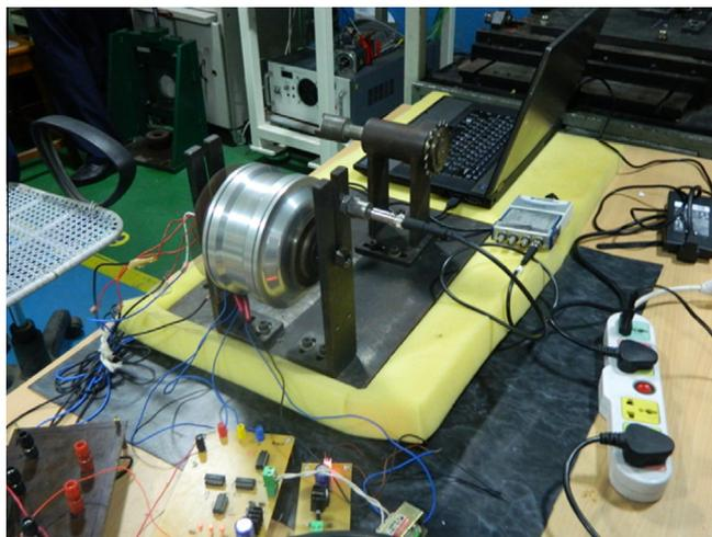
**Fig. 26.** Experimental setup to measure vibration.
