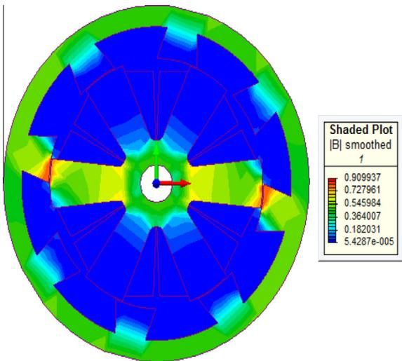
Fig. 4. Flux density plot in an intermediate position.
