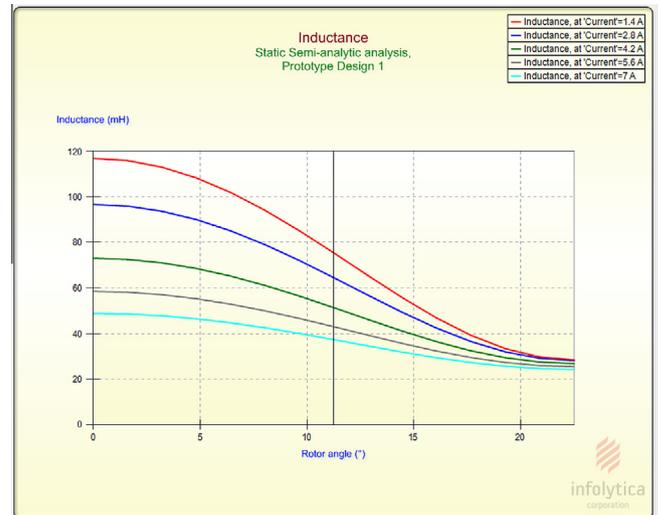
Fig. 6. Inductance profile of 6/8 pole SRHM.
