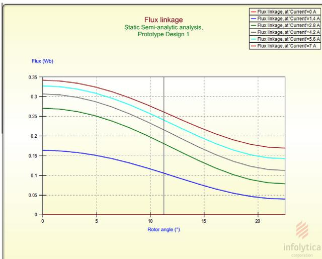
Fig. 5. Current - flux linkage characteristics.
