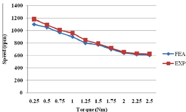
Fig. 18. Comparison of FEA and test data.
