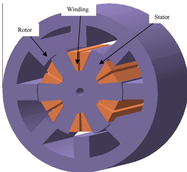
Fig. 1. Two dimensional view of SRHM.
