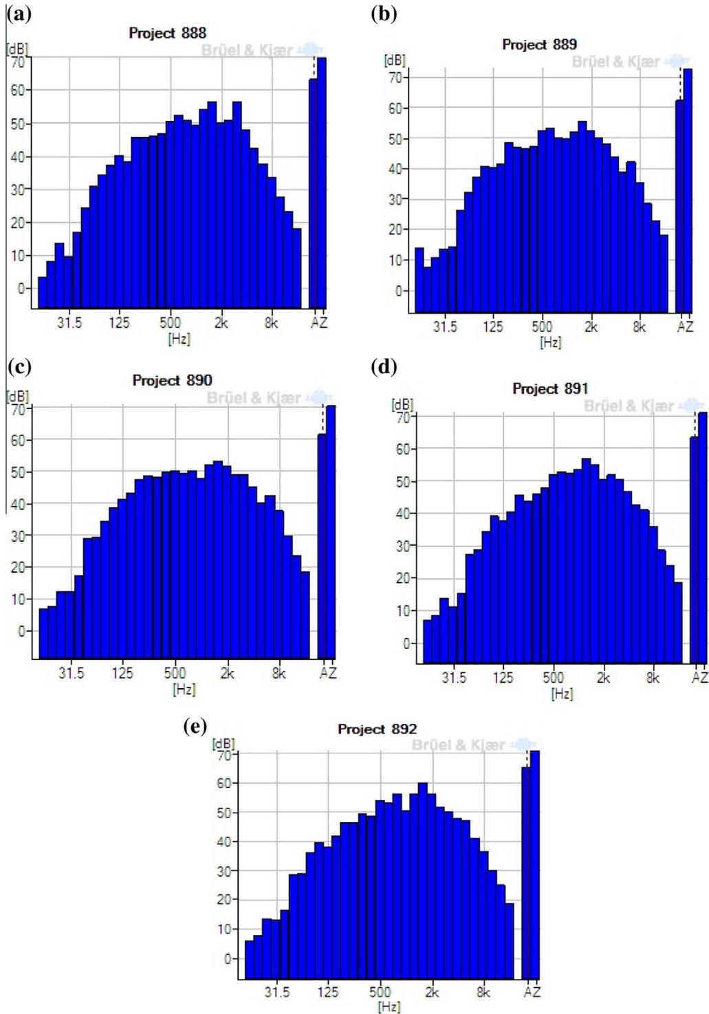
Fig. 32. Noise spectrum for the speed of 1000 RPM at (a) shaft position (b) right side (c) left side (d) opposite to shaft position (e) top position.
