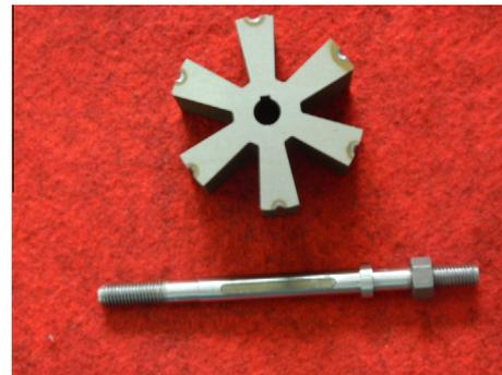
Fig. 12. Stator lamination and shaft with key.
