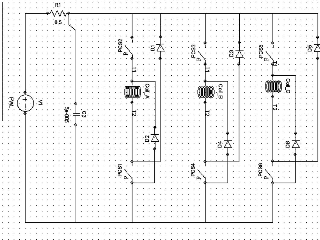
Fig. 8. Three phase model of the SRHM converter in circuit domain.
