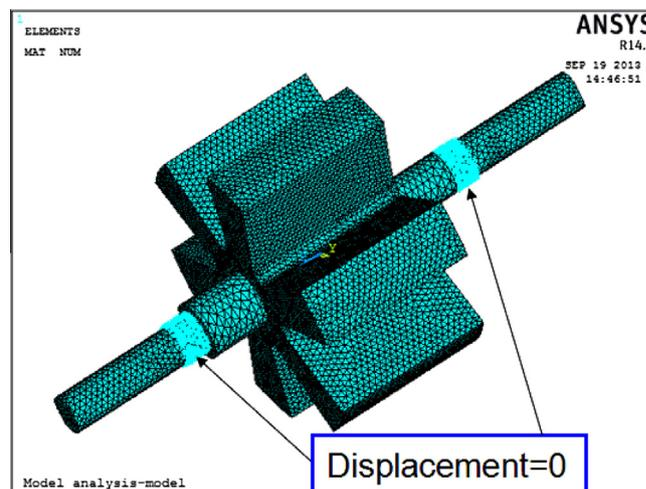
Fig. 19. 3D model with boundary condition.
