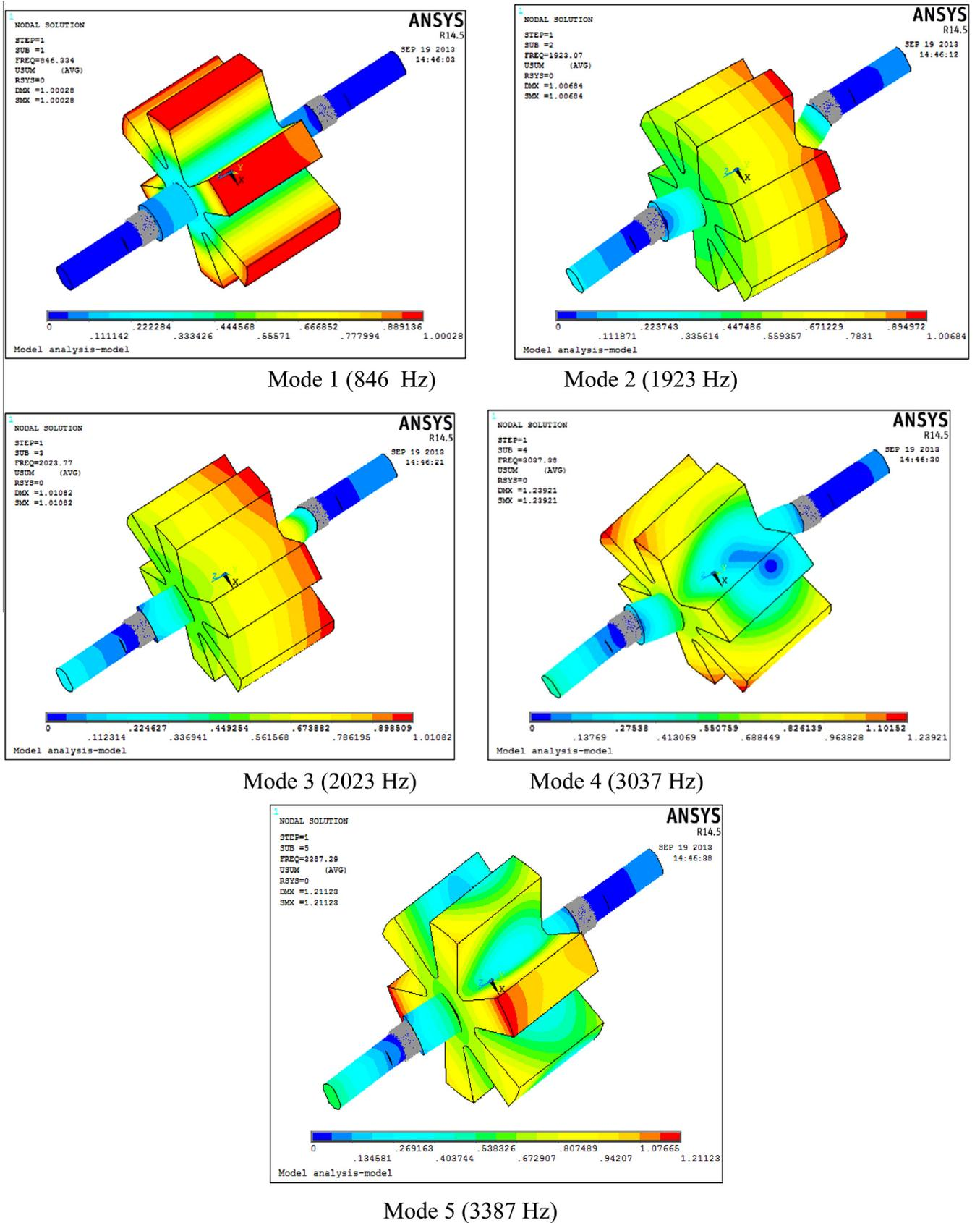
Fig. 20. Stator mode shape using 3-D analysis.
