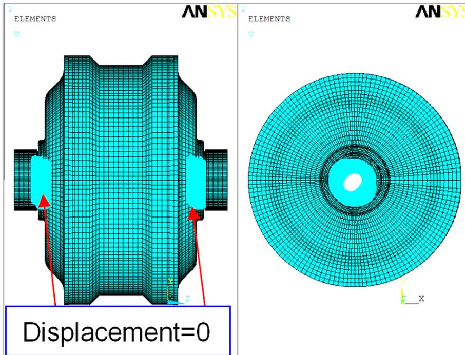
Fig. 21. Meshed model and boundary conditions.
