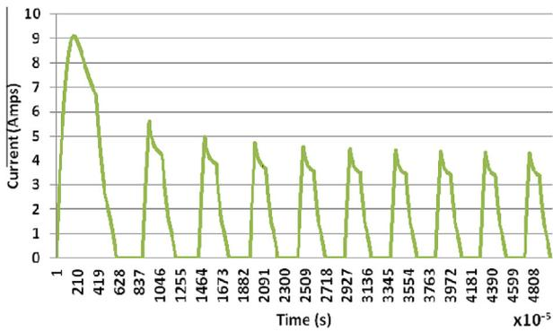
Fig. 9. Current waveform of phase A at 0.75 N m.
