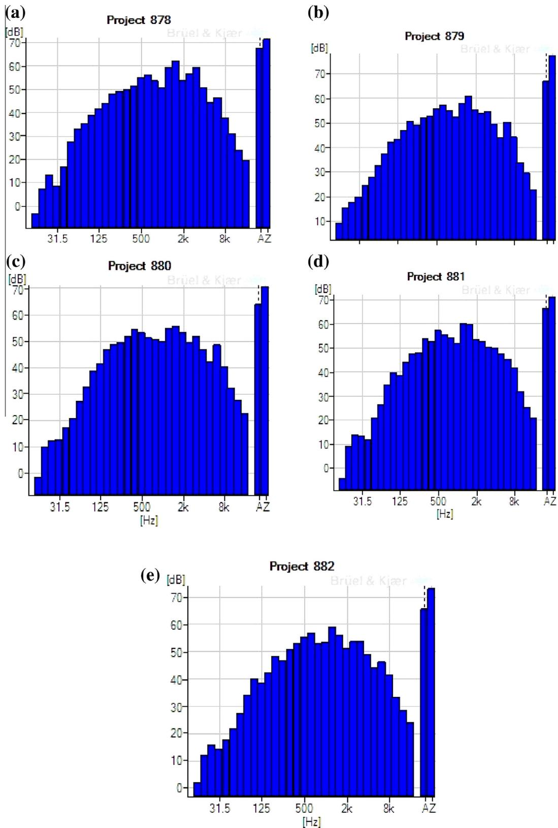
Fig. 30. Noise spectrum for the speed of 500 RPM at (a) shaft position (b) right side (c) left side (d) opposite to shaft position (e) top position.
