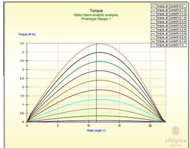
Fig. 7. Single phase torque profile at different currents.
