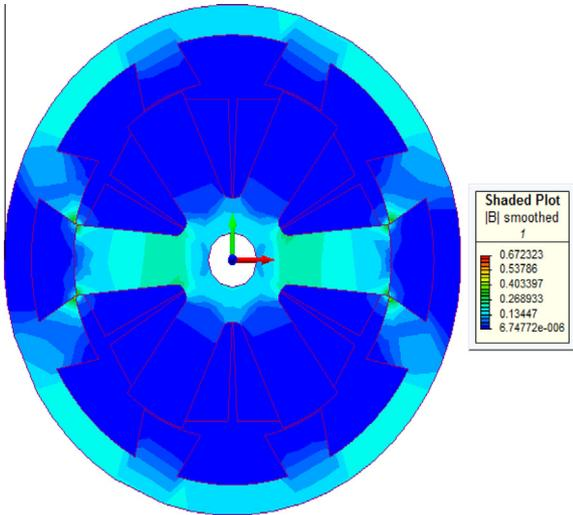
Fig. 3. Flux density plot in the unaligned position.
