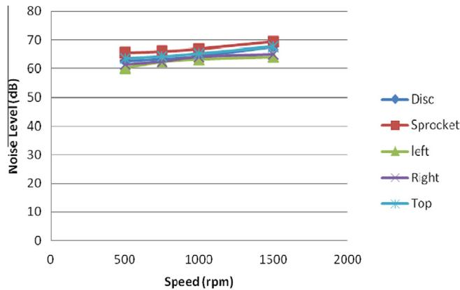
Fig. 33. Measurement of noise level in SRHM.
