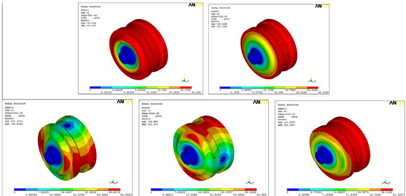
Fig. 22. Rotor assembly mode shapes and modal frequencies.
