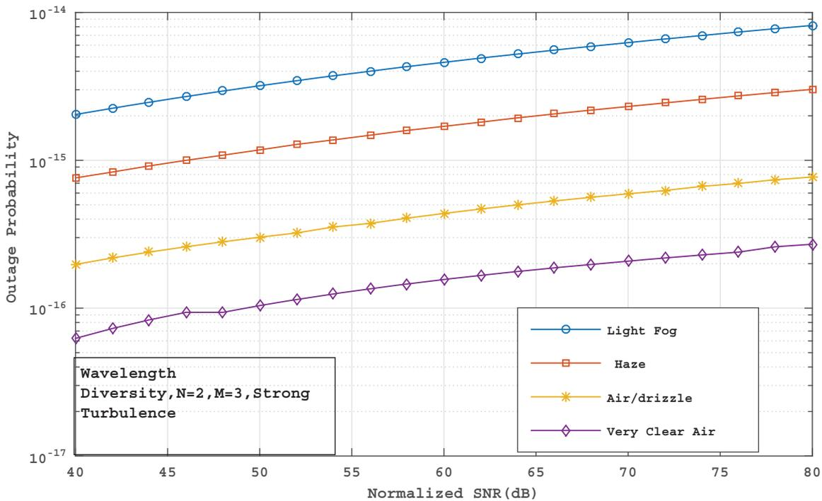
Figure 7: outage probability of multi-hop parallel FSO system for Wavelength diversity case using M distribution model for the case of strong turbulence including weather conditions.
