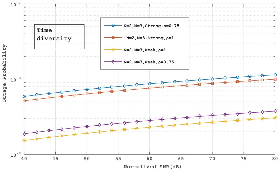
Figure 5: Outage probability of multi-hop parallel FSO system for Time diversity case using M distribution model for the case of both weak and strong turbulence conditions.
