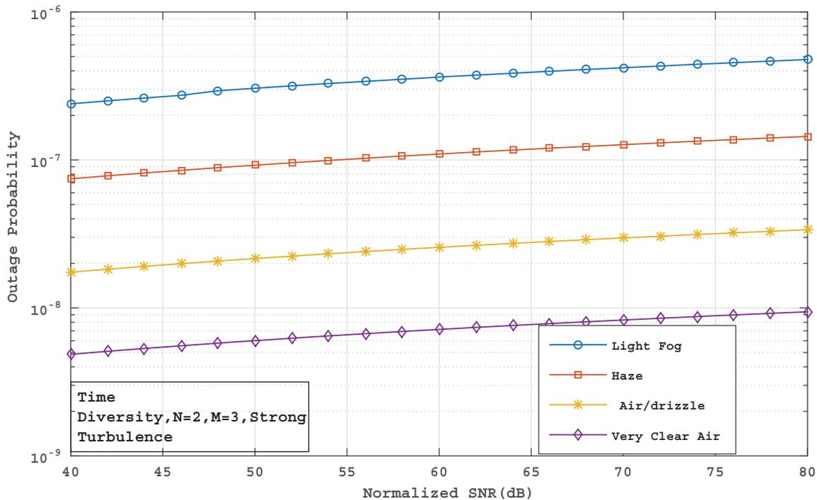
Figure 8: Outage probability of multi-hop parallel FSO system for Time diversity case using M distribution model for the case of strong turbulence including weather conditions.
