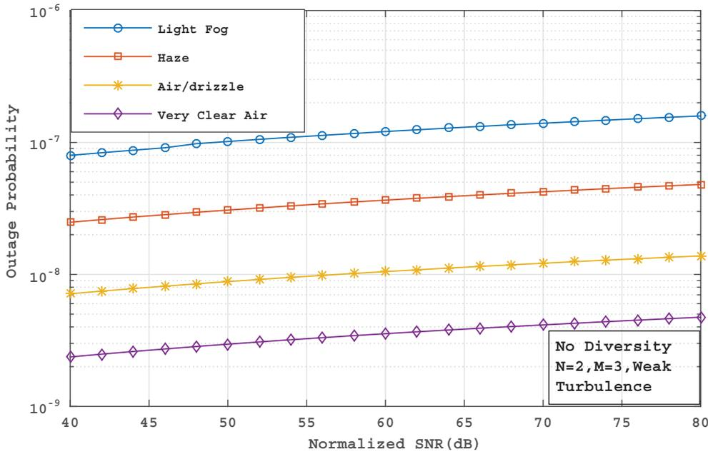
Figure 6: Outage probability of multi-hop parallel FSO system for No diversity case using M distribution model for the case of weak turbulence including weather conditions.
