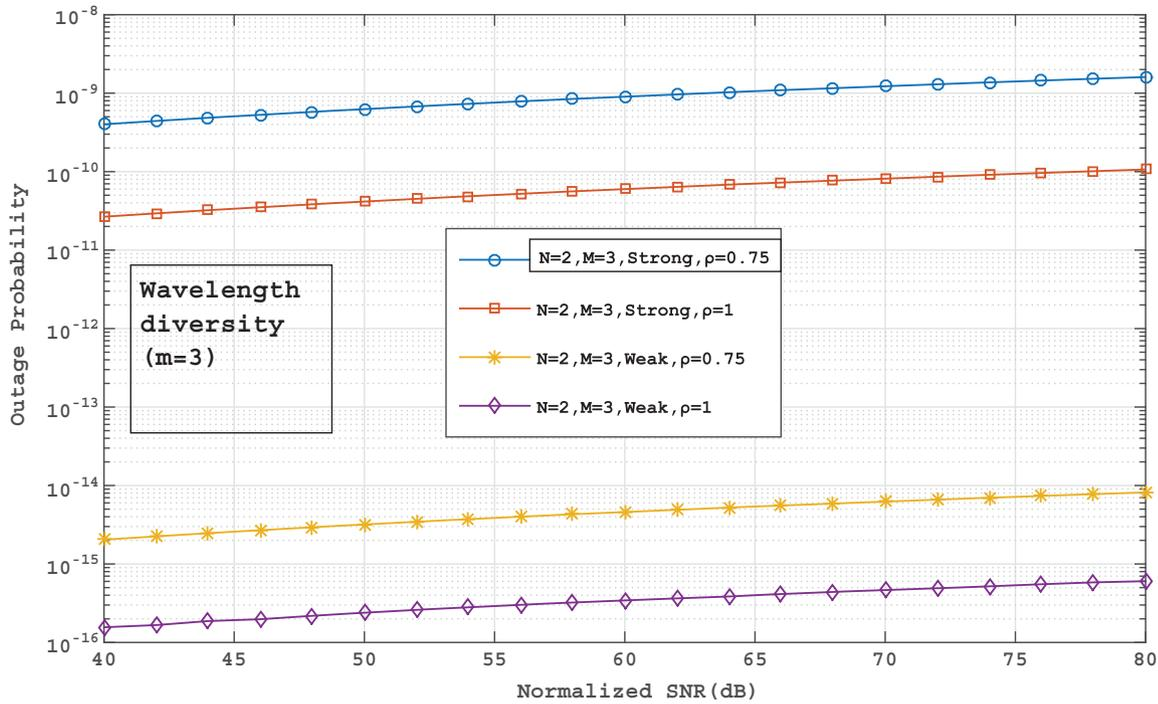
Figure 4: Outage probability of multi-hop parallel FSO system for wavelength diversity case using M distribution model for the case of both weak and strong turbulence conditions [ $m = 3$ ].
