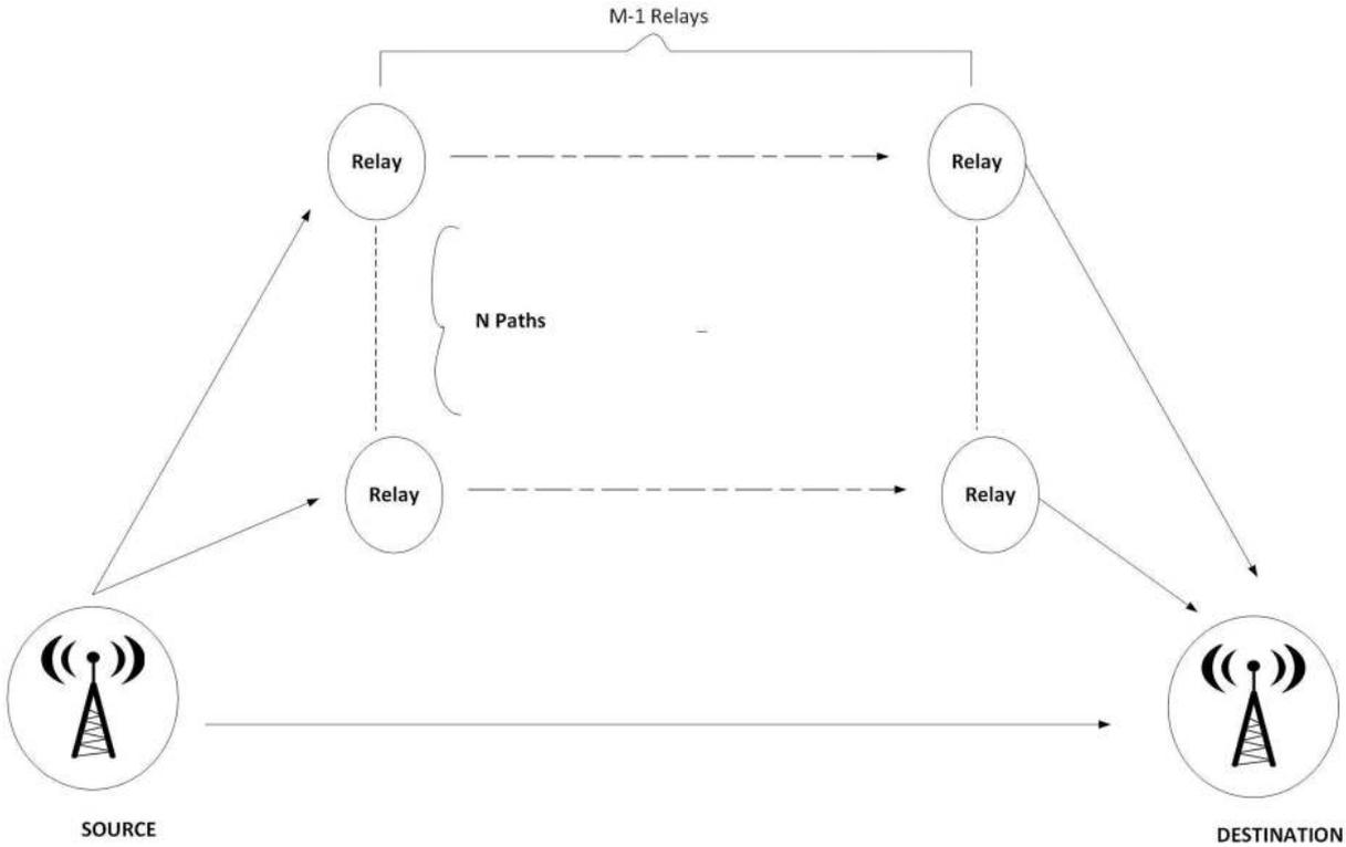
Figure 1: Schematic of Multi-hop DF FSO system.
