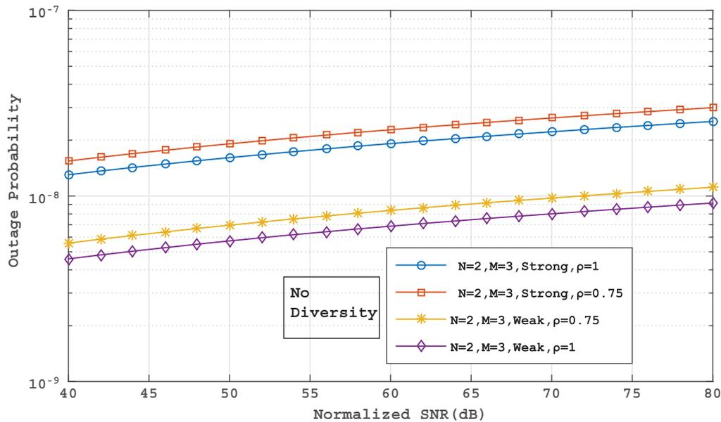
Figure 3: Outage probability of multi-hop parallel FSO system for no diversity case using M distribution model for the case of both weak and strong turbulence conditions.
