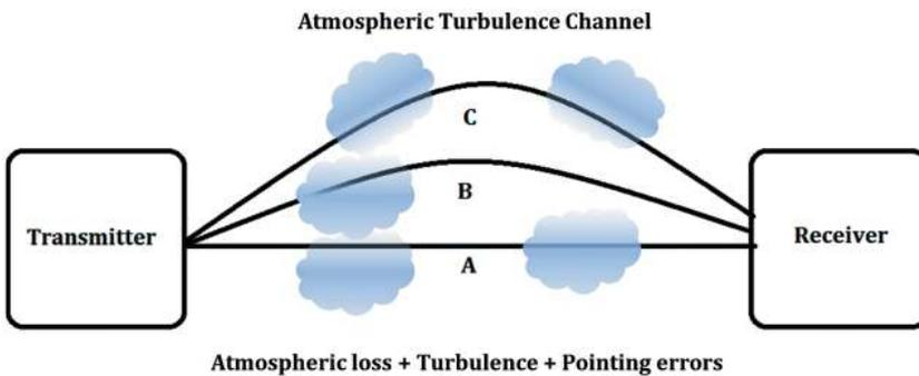
Figure 2: Optical signal transmission in wireless communication system [16].
