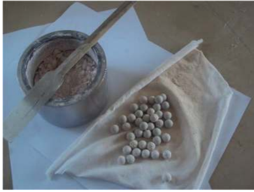
FIGURE 1: Zirconium balls and metakaolin during grinding.
