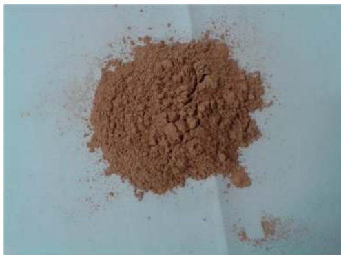
FIGURE 4: Ultrafine ceramic powders after grinding in a planetary ball.
