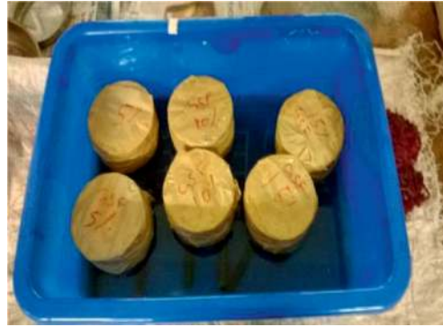
FIGURE 6: Specimens for the sorptivity test.
