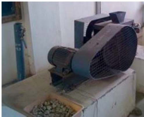
FIGURE 3: Jaw crusher for crushing tiles.
