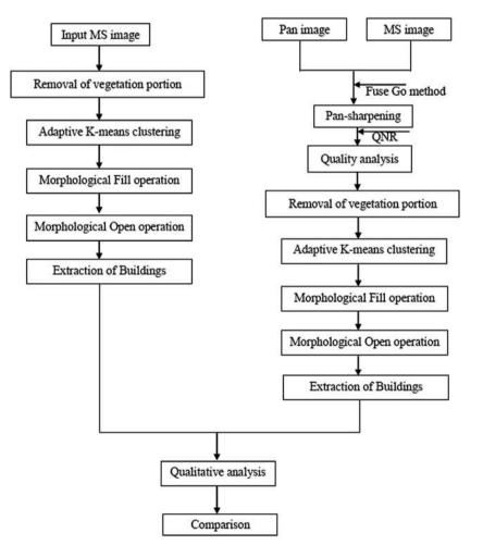
Figure 3. Methodology for extracting the building manually.
