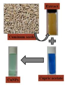
Figure 1. Schematic synthesis procedure of bio-CuNPs using *Cuminum cyminum* seed extract.
