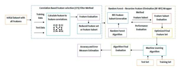
Figure 3. Architecture diagram of proposed hybrid CFS and RF-RFE feature selection approach.
