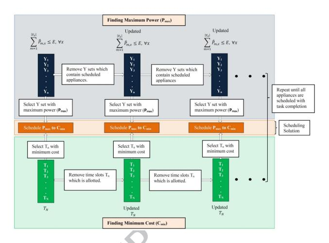
Fig. 2. Proposed Minimum Cost Maximum Power (MCMP) algorithm
