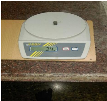
Figure 4. Measurement of Sintered Weight
