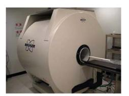
FIGURE 1: 7 T Bruker Avance magnet.
