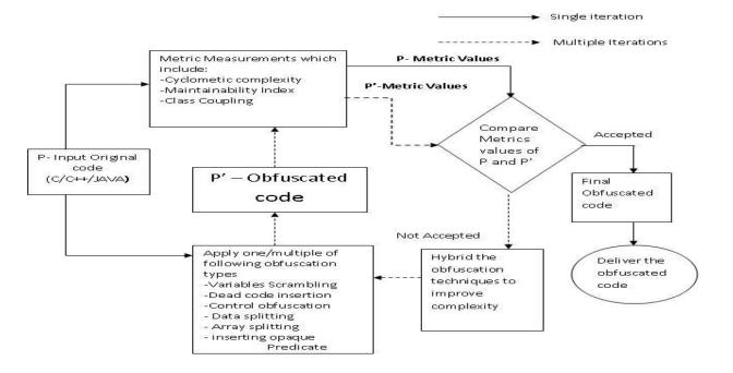
Figure 1 Propose Block diagram - M-COT (Metrics based Code Obfuscation Techniques)
