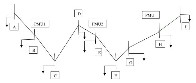
Figure 1. Complete observability using PMU's
