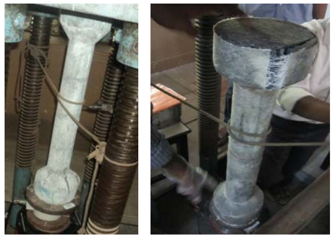
FIGURE 4: Failure crack pattern (before and after wrapping).
