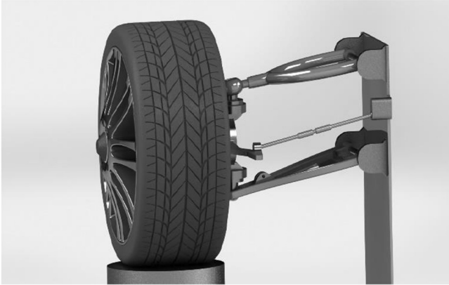
Fig. 4. SOLIDWORKS model of the setup with variable length upper arm and tie rod.
