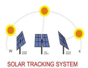
Figure 2. Solar Tracking Mechanism
