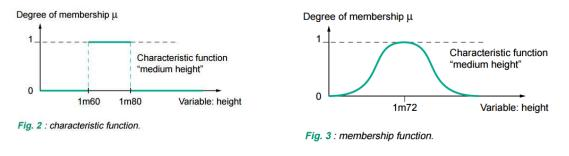
Figure 2. Characteristic Function
