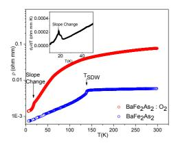
**FIGURE 2.** The results of resistivity vs temperature measurement for BaFe<sub>2</sub>As<sub>2</sub>:O<sub>2</sub> and BaFe<sub>2</sub>As<sub>2</sub>.Inset shows  $d\rho/dT$  vs T for BaFe<sub>2</sub>As<sub>2</sub>:O<sub>2</sub>.
