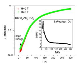
**FIGURE 3.** The results of resistivity vs temperature measurement for  $BaFe_2As_2:O_2$  at H = 0 and 5 T. The inset shows MR as a function of temperature.
