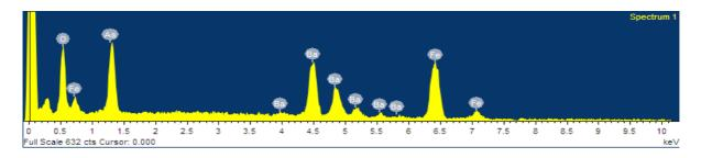
**FIGURE 1.** The results of E DAX measurements of  $BaFe_2As_2$  single crystals which were kept in air ambience for several months.
