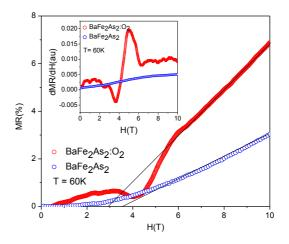
**FIGURE 4.** MR vs H for BaFe<sub>2</sub>As<sub>2</sub>:O<sub>2</sub> and BaFe<sub>2</sub>As<sub>2</sub>, shown in positive direction, displayed at a representative temperature 60K. The straight line guides the eye for the linear region. The inset shows dMR/dH vs H for both.
