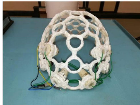
FIGURE 5. EEG sensor manufactured with 16 electrodes.
