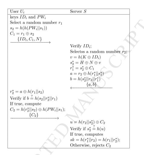
Figure 2: Login and authentication phase of Lee et al. scheme[19].
