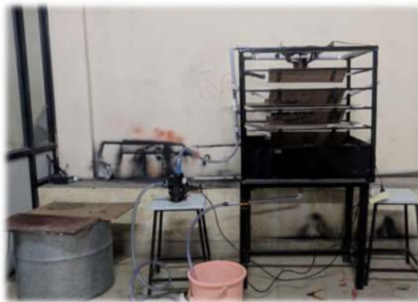
Figure 2. Experimental setup (Cooling Tower)
