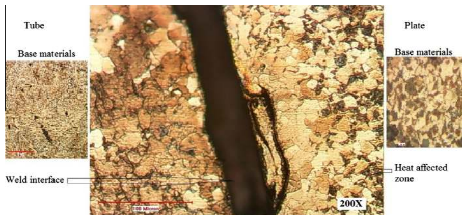
Figure A.21 Microstructure of the workpiece with steel ball (1800 rpm).
