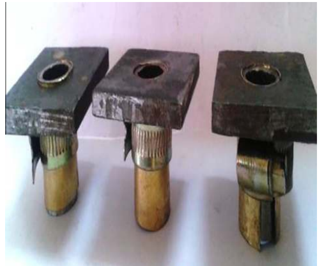
Figure A.6 Three sets of workpiece with brass sheet.
