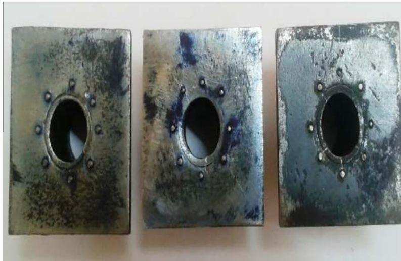
Figure A.9 Three sets of workpiece with steel ball before welding.
