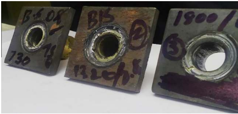
Figure A.13 Workpiece after welding with bronze sheet.
