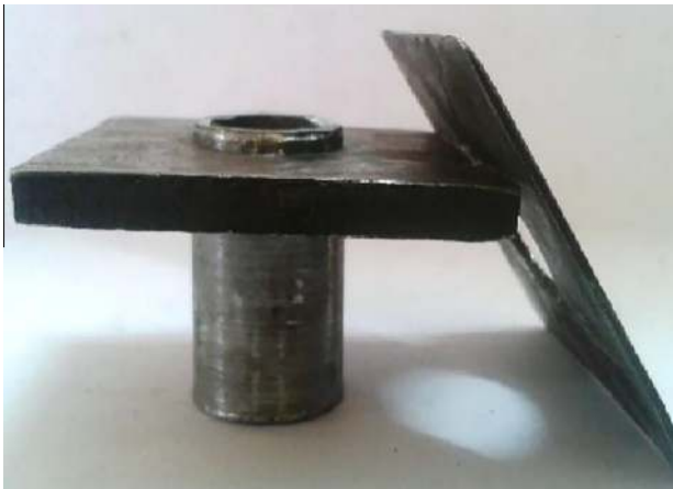
Figure A.3 Workpiece with filler plate SA 387.
