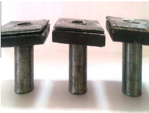
Figure A.4 Three sets of workpiece with filler plate and tube projection.
