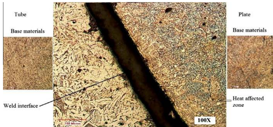
Figure A.20 Microstructure of the workpiece with filler plate (1800 rpm).
