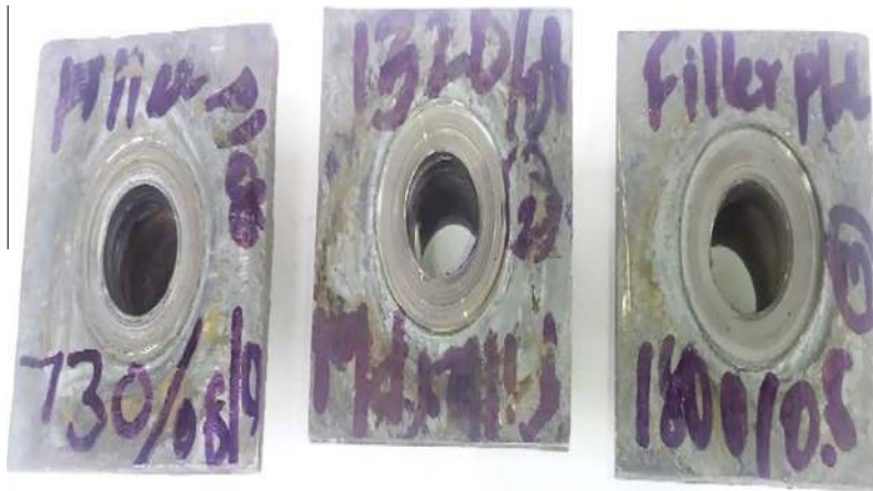
Figure A.14 Workpiece after welding with filler plate.
