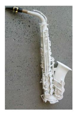
Fig. 2 Additive-manufactured Saxophone. Source [11]
