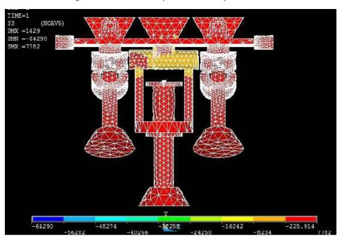
Fig.8. Mechanical stress intensity on the hub of screwjack mechanism
