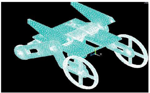
Fig.6. Meshed sequence of wheelchair
