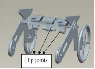
Fig.1. Wheelchair base interfaced with hip joints.
