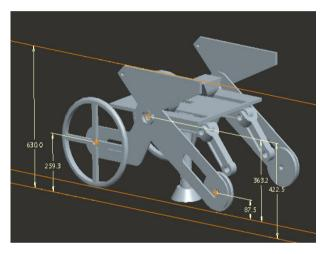
Fig.3. Solid model of the wheel chair and leg assembly with dimensions
