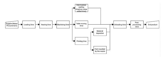
Figure7illustrates the time-consuming process involved in additive manufacturing
