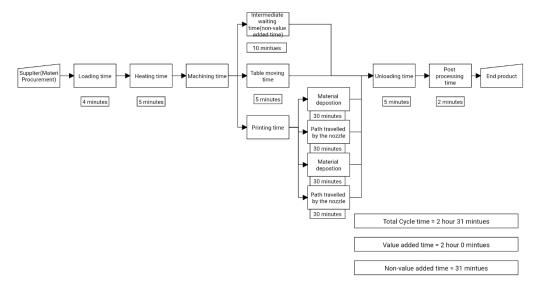
Value stream mapping of printing grouped sample models simultaneously:
