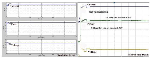
Fig. 2 Simulated and experimental results of voltage, current, and power tracked for modified PSO algorithm under constant irradiation condition
