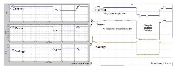
Fig. 3 Simulated and experimental results of voltage, current, and power tracked using modified PSO algorithm for variation in irradiation condition
