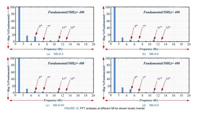
The variation of the parameters like modulation index and THD with harmonic spectrum is compared with various topologies and is represented in Table III. It is found that the THD of the proposed topology holds the best in its outcome with a lesser value. The harmonic spectrum at different modulation index are shown in Fig 12.
