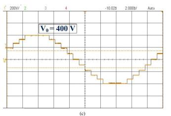
FIGURE 16. The experimental output voltage of (a) seven (b) nine (c)
