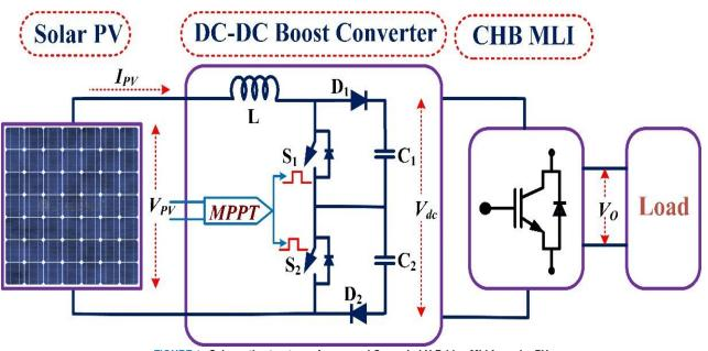
FIGURE 1. Schematic structure of proposed Cascaded H Bridge MLI for solar PV
