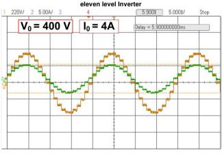
FIGURE 17. Experimental output voltage and current of eleven level Inverter
