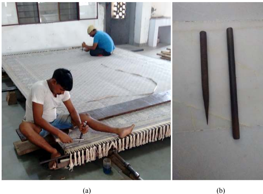
Figure 1 (a) A typical postural position adapted to perform carpet alignment and (b) conventional chisel and hammering rod (see online version for colours)
