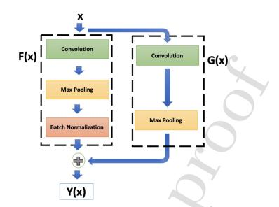
Fig. 2. A representation of the functions F(x) and G(x) that are skipped through the RPFE block to generate the output Y(x) from the residual block.
