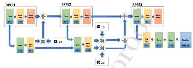
Fig. 3. An overview of the architecture employed to integrate attention within the residual net framework.
