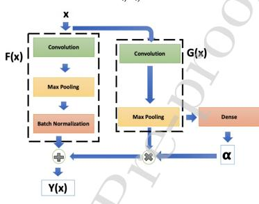
Fig. 4. A visual representation for generating the output Y(x) from an ARPFE block using attention based weights.
