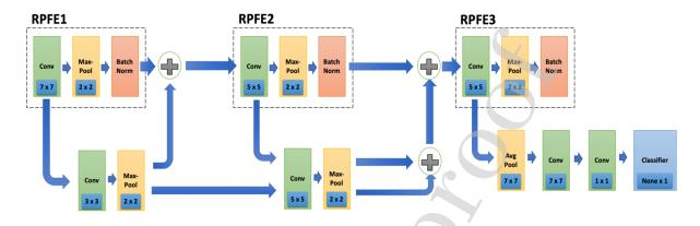
Fig. 1. The architecture of the Proposed Residual CNN
