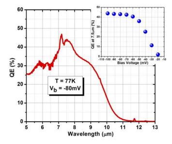
FIG. 2. Saturated quantum efficiency spectrum of the device at -80 mV applied bias voltage in front-side illumination configuration without any anti-reflection coating. Inset: Quantum efficiency of the device at 7.5  $\mu$ m in front-side illumination configuration as a function of applied bias voltage (V<sub>b</sub>).
