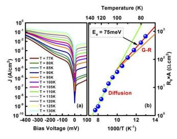
FIG. 3. (a) Dark current density *vs.* applied bias voltage characteristic of the sample as a function of temperature. (b)  $R \times A$  *vs.* 1/T; the sample exhibited an Arrhenius type behavior with an associated activation energy (E<sub>a</sub>) of about ~75 meV below 100 K. At temperatures above 100 K, the device dark current is completely diffusion-limited. The green and orange lines represent the expected diffusion and generation-recombination (G-R) limits, respectively.
