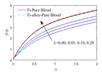
**Fig. 9** Effect of  $\lambda$  on dimensionless stream function
