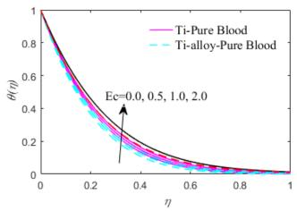
**Fig. 29** Effect of Ec on temperature profile
