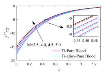
**Fig. 7** Effect of *M* on shear stress
