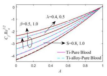
**Fig. 30** The variation of skin friction coefficient against first order velocity slip, Casson fluid, suction, ratio parameters.
