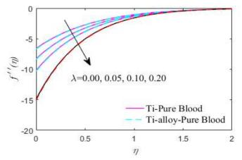
**Fig. 11** Effect of  $\lambda$  on shear stress
