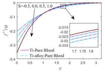
**Fig. 23** Effect of *S* on shear stress
