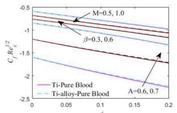
**Fig. 31** The variation of skin friction coefficient against magnetic, Casson fluid, volume fraction and ratio parameters.
