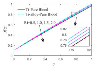
Fig. 17 Effect of Ri on dimensionless stream function
