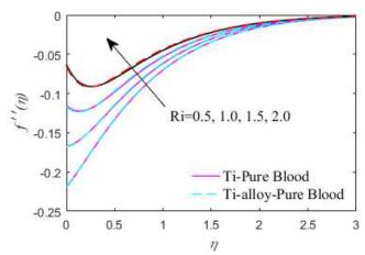
Fig. 19 Effect of Ri on shear stress
