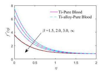
**Fig. 14** Effect of  $\beta$  on velocity profile
