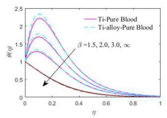
**Fig. 16** Effect of  $\beta$  on temperature profile
