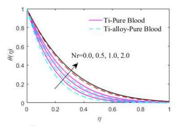
**Fig. 28** Effect of Nr on temperature profile
