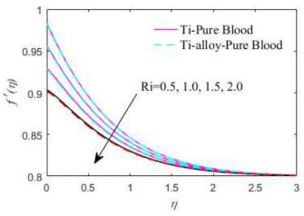
Fig. 18 Effect of Ri on velocity profile
