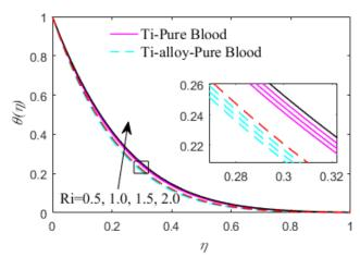
**Fig. 20** Effect of *Ri* on temperature profile
