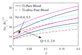
Fig. 32 The variation of Nusselt number against heat source, volume fraction and radiation conduction parameter
