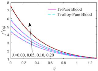
**Fig. 10** Effect of  $\lambda$  on velocity profile
