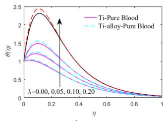
**Fig. 12** Effect of  $\lambda$  on temperature profile
