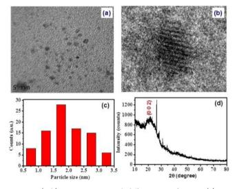
**Figure 1.** (a, b) HRTEM image with different magnifications, (c) size distribution chart for CQDs, and (d) XRD pattern of CQDs.
