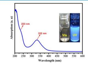
Figure 4. UV-visible absorption spectrum of CQDs.
