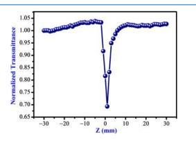
Figure 9. Open aperture Z-scan pattern of as-prepared CQDs.
