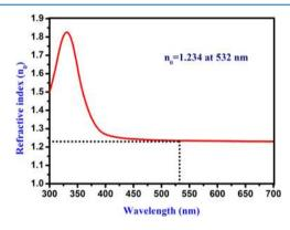
Figure 5. Linear refractive index of carbon quantum dots.
