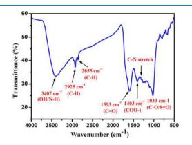
Figure 2. FTIR spectrum of synthesized CQDs.
