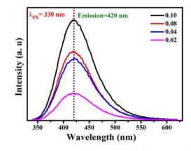
Figure 6. Fluorescence emission spectrum of CQDs at different concentrations.
