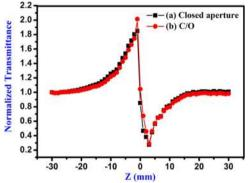
**Figure 8.** (a) Closed and (b) ratio of closed and open aperture *Z*-scan patterns of as-prepared CQDs.
