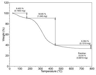
Fig. 5. Thermogravimetric analysis of synthesized ZnO NPs
