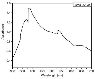
Fig. 1. UV-visible spectrum of zinc oxide nanoparticles
