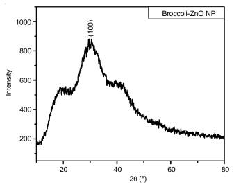
Fig. 2. XRD spectra of B. oleracea extract synthesized ZnO nanoparticles
