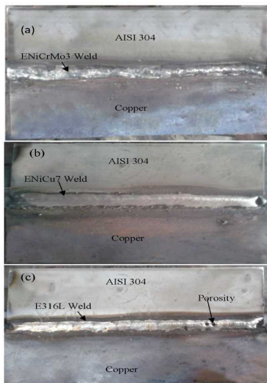
Fig. 1. As welded sample of AISI 304- CP copper using three different filler materials, (a)ENiCrMo3, (b)ENiCu7 and (c)E316L
