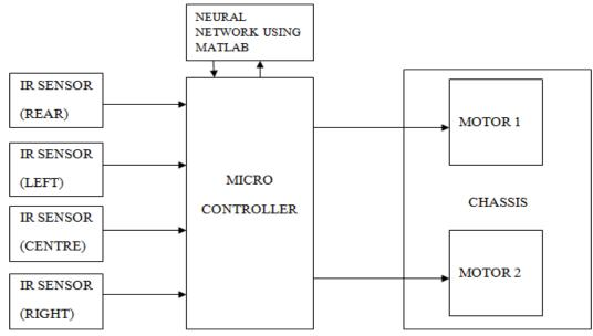
Figure 2. Block diagram of the proposed system
