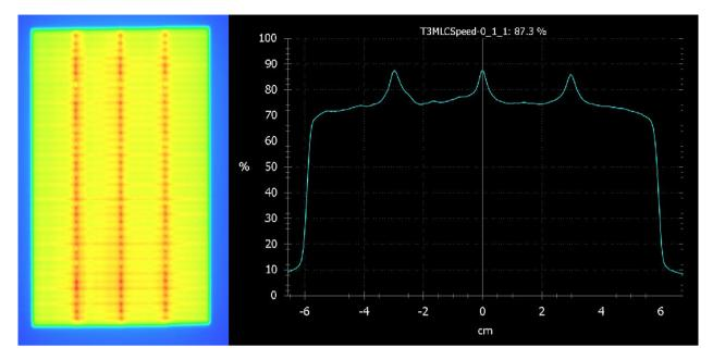
Fig. 16 – The image obtained on EPID and evaluated using the Portal Dose Prediction Software to evaluate accurate control of leaf speed during RapidArc delivery.
