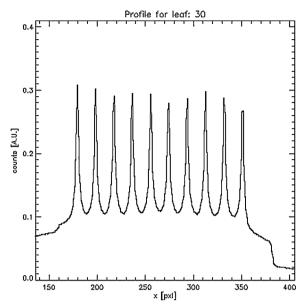
Fig. 9 – The image obtained for the picket fence test at a stationary angle and during gantry rotation on EPID and evaluated using the EPIQA.
