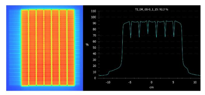
Fig. 14 – The image taken on EPID and evaluated using the Portal Dose Prediction Software to evaluate accurate control of dose rate and gantry speed during RapidArc delivery. Even the portal dose shows equal exposures in all strips.
