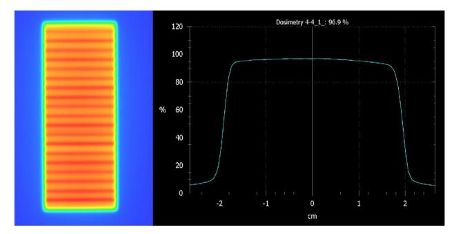
Fig. 4 - Result obtained for dosimetric test from portal dosimetry.
