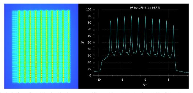
Fig. 6 – The image obtained for the picket fence test at a stationary angle on a EPID and evaluated using the Portal Dose Prediction Software.
