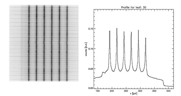
Fig. 12 – The image obtained for the picket fence test with a sub millimeter error introduced taken on EPID and evaluated using the EPIQA. Intentional errors introduced in the picket fence pattern were clearly noticeable.
