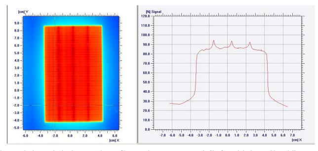
Fig. 15 - The image obtained on EDR2 therapy film to evaluate accurate control of leaf speed during RapidArc delivery.
