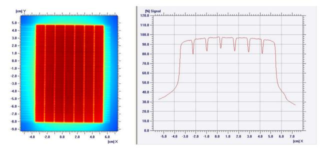
Fig. 13 – The image taken on EDR2 therapy film to evaluate accurate control of dose rate and gantry speed during RapidArc delivery. All the strips show equally exposed regions when evaluated with Omnipro software.
