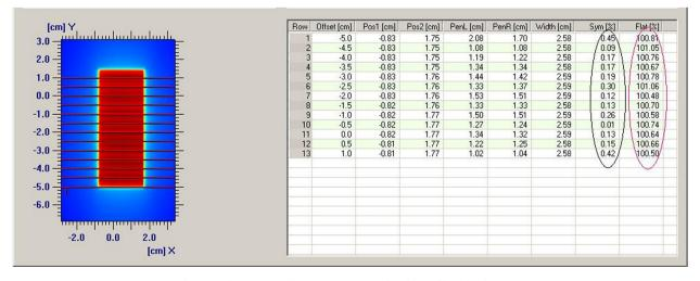
Fig. 2 - Flatness and symmetry results from film dosimetry.
