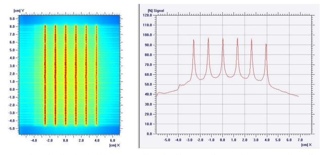
Fig. 10 – The image obtained for the picket fence test with a sub millimeter error introduced taken on EDR2 therapy film. The planned error is exactly observed in the image.
