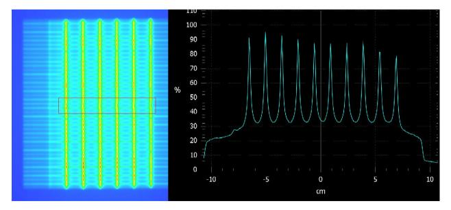
Fig. 11 – The image obtained for the picket fence test with a sub millimeter error introduced taken on EPID and evaluated using the Portal Dose Prediction Software. As seen above the portal dose image also shows the sub millimeter error introduced in the MLC position.
