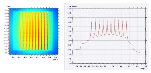
Fig. 7 - The image obtained for the picket fence test at a stationary angle and during gantry rotation on a EDR2 therapy film.
