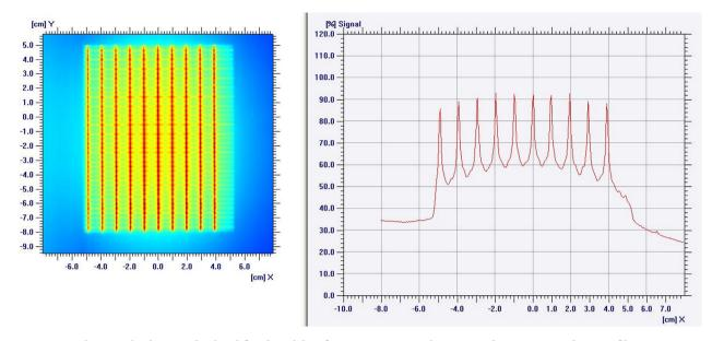
Fig. 5 - The image obtained for the picket fence test at a stationary angle on a EDR2 therapy film.
