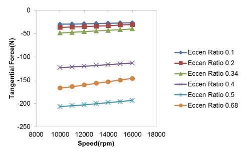
Fig. 10. Tangential force vs speed for helically-grooved labyrinth seal
