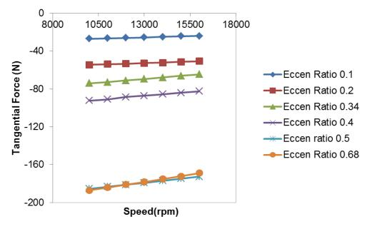
Fig. 11. Tangential force vs speed for circumferentially-grooved labyrinth seal
