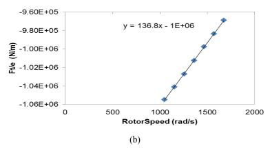
Fig. 5. Seal forces versus rotor speed in (a) Radial direction (b) Tangential direction
