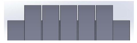
Fig. 3. 2D view of circumferentially-grooved labyrinth seal
