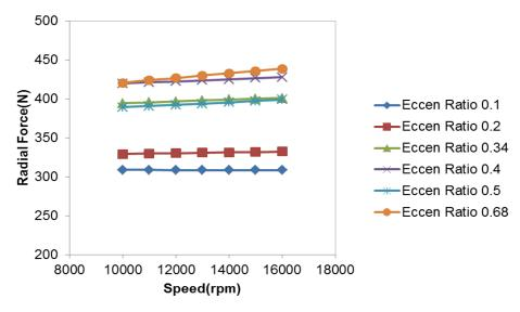
Fig. 8. Radial forces vs speed for helically-grooved labyrinth seal
