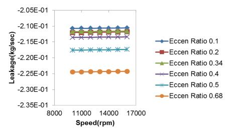
Fig. 7. Leakage vs speed for circumferentially-grooved labyrinth seal
