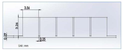
Fig. 1. Dimensions of labyrinth seal
