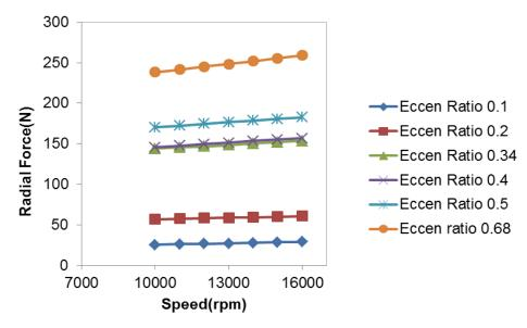
Fig. 9. Radial force vs speed for circumferentially-grooved labyrinth seal
