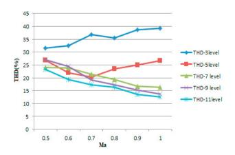
Fig.10 THD Vs Ma of 3, 5, 7, 9 and 11 level Inverter
