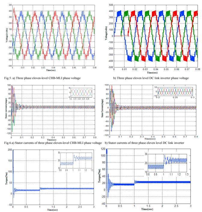
Fig.7.a) Variation in torque of 11-level cascaded fed induction motor drive b) Variation in Torque of three phase eleven level DC link inverter
