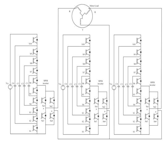
Fig.2 Eleven level DC link inverter fed induction motor drive with reduced switches
