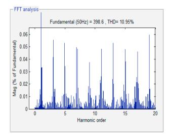
Fig.9.a) THD spectrum of 11-level CHBMLI fed induction motor drive b) THD spectrum of eleven level DC link inverter fed induction motor
