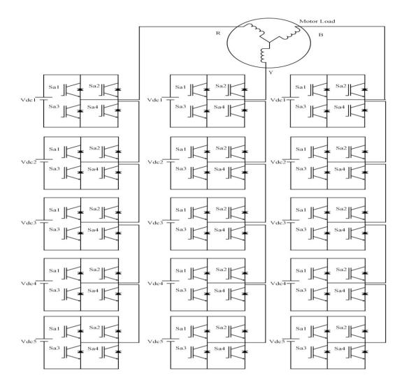
Fig.1. Three-phase eleven level cascaded inverter fed induction motor drive
