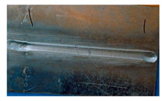
Figure 1. Bead appearance of TIG welding.
