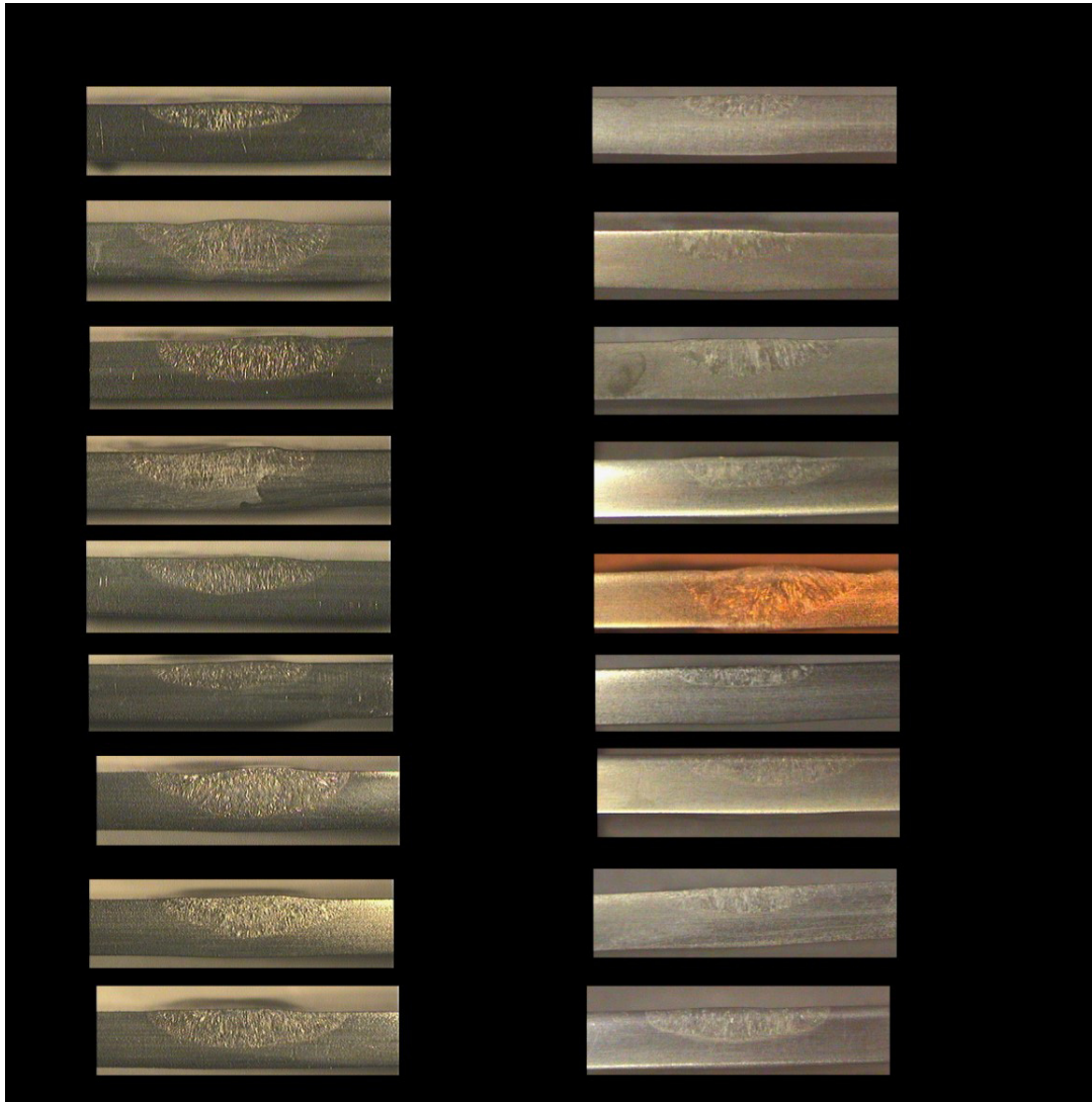
Fig. 1 Macrograph and Bead profile of high frequency and low frequency PCGTAW with penetration (P) in mm, width (W) in mm, depth to width ratio (W/P) and heat input (HI) J/mm.
