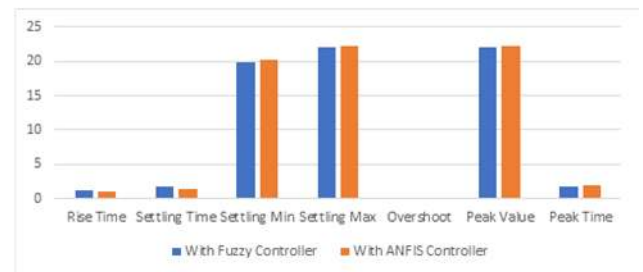
FIGURE 29. Step response comparison chart of 31-level cascaded inverter with controllers.
