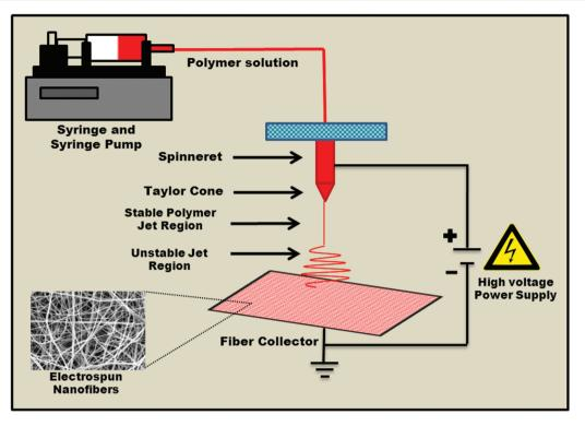
Figure 1. Schematic illustration of the electrospinning setup and process conditions.
